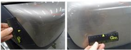
Roof, Scratch(es), LI - Repair and paint (complete)
