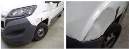
Bonnet, Dent(s), LI - Repair and paint (complete)
