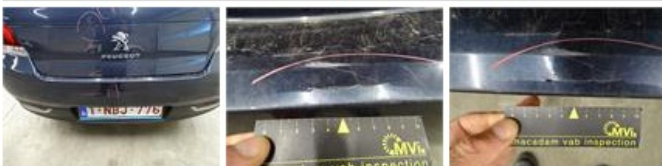
Bumper R, Dent(s) and scratch(es), LI - Repair and paint (complete) 211,80
