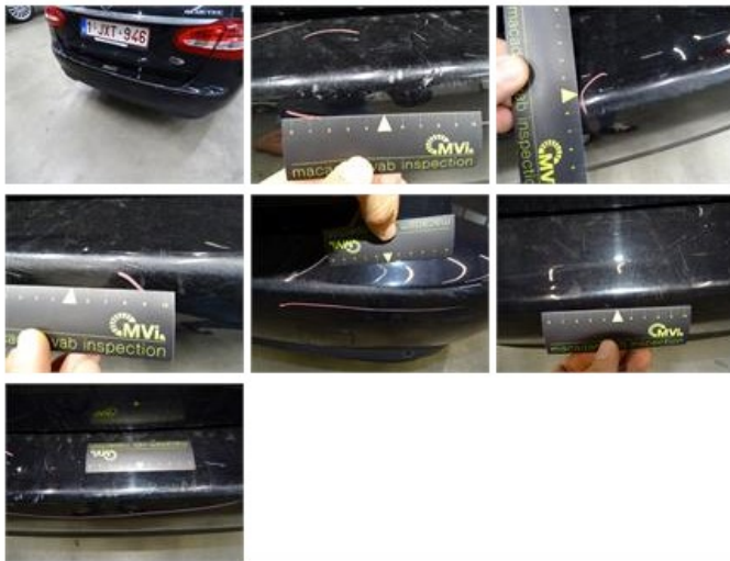
Wing R R, Dent(s) and scratch(es), LI - Repair and paint (partial)
