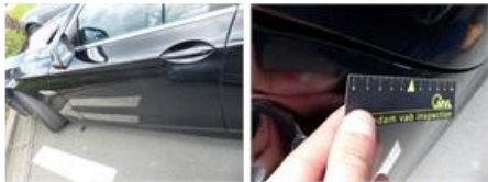
Wing F R, Deformed / Strained, Repair/replace (lump sum)
