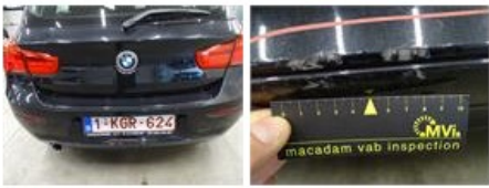
Roof, Dent(s), LI - Repair and paint (complete)
