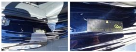
Roof, Scratch(es), LI - Repair and paint (complete)
