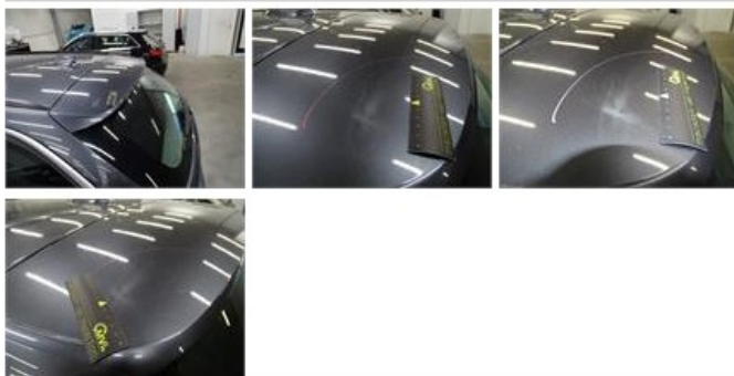
Roof, Scratch(es), LI - Repair and paint (complete)
