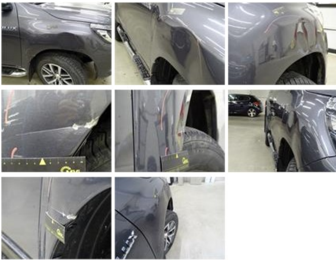
Bumper corner R R, Deformed / Strained, Smart repair
