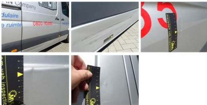
Sliding door R, Deformed / Strained, Le - Replace and paint
