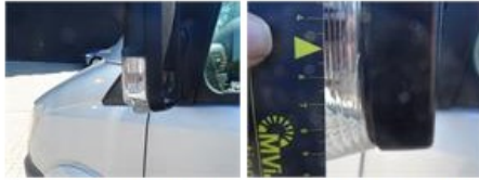
Sliding door R, Dent(s) and scratch(es), LI - Repair and paint (complete)
