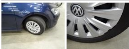
Wheel cover F L, Broken, E - Replace
