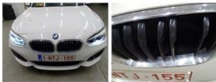
Bumper grille F L, Broken, E - Replace
