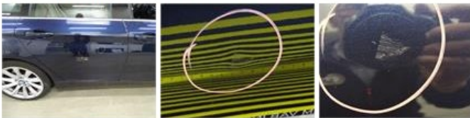
Door R R, Dent(s) and scratch(es), LI - Repair and paint (complete) 0,00
