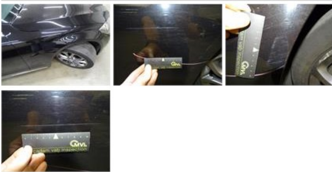
Door R R, Scratch(es), LI - Repair and paint (complete)
