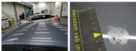
Tailgate, Scratch(es), LI - Repair and paint (complete)
