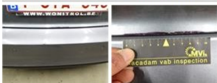
Tailgate, Scratch(es), LI - Repair and paint (complete)
