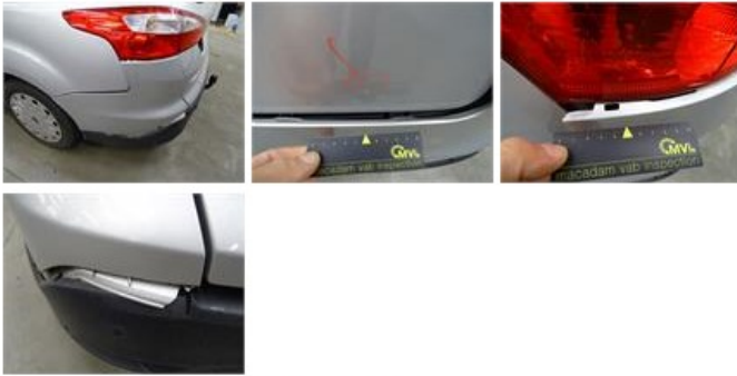
Wing F R, Dent(s), LI - Repair and paint (complete) 220,18
