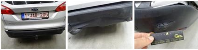
Bumper R, Deformed / Strained, E - Replace 415,20
