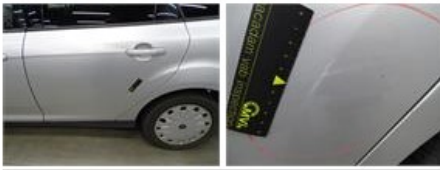
Bumper corner R R, Deformed / Strained, Smart repair 110,64
