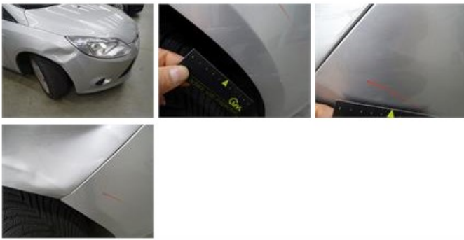
Bumper corner R R, Deformed / Strained, Smart repair 110,64
