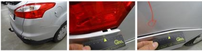
Door R L, Scratch(es), LI - Repair and paint (complete) 318,35
