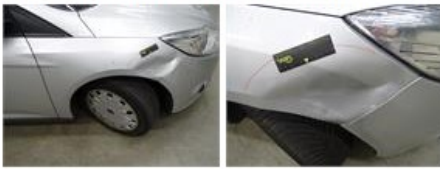
Bumper R, Deformed / Strained, E - Replace 415,20
