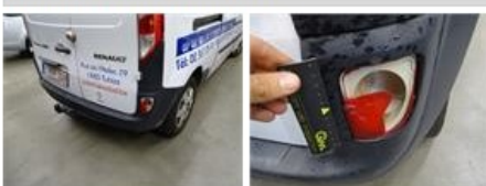
Reflector, Broken, E - Replace
