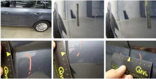
Door R L, Bad repair, LI - Repair and paint (complete)
