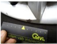
Door R R, Dent(s) and scratch(es), Le - Replace and paint
