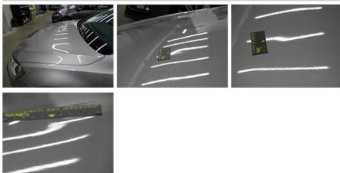
Roof, Chemical polution, LI - Repair and paint (complete)
