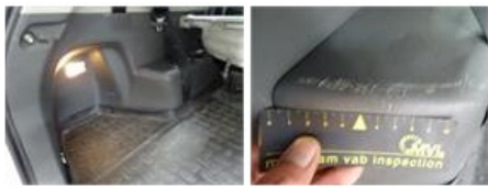
Sill outer R, Scratch(es), It - Spot repair
