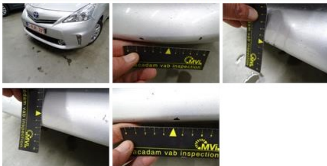
Door panel R L, Hole, Smart repair
