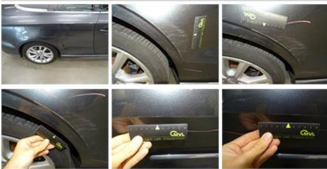
Sill outer R, Scratch(es), LI - Repair and paint (complete)
