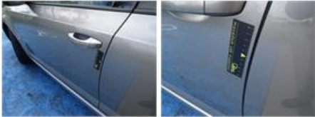
Door R R, Bad repair, LI - Repair and paint (complete)
