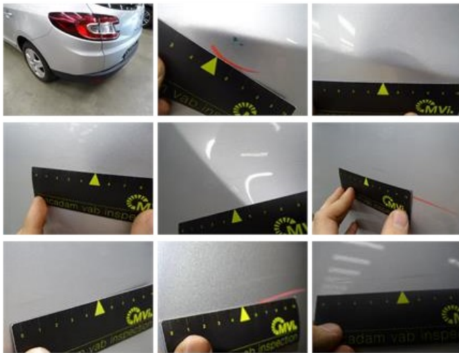
Bumper corner R R, Scratch(es), Acceptable
