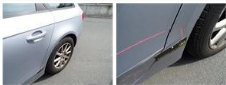
Sill outer R, Dent(s) and scratch(es), Le - Replace and paint
