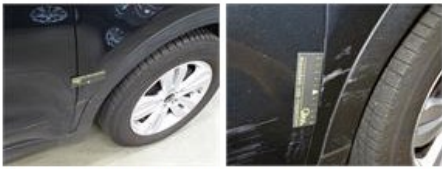
Door F R, Deformed / Strained, Le - Replace and paint
