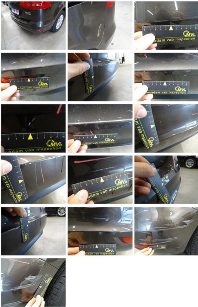
Protection plate M, Hole, E - Replace
