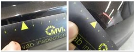
Roof pillar L, Chemical polution, LI - Repair and paint (complete)
