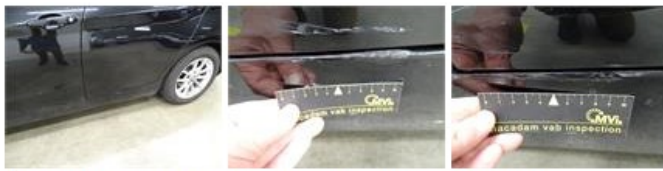
Door R L, Dent(s) and scratch(es), LI - Repair and paint (complete)
