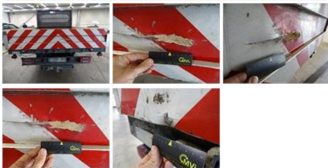
Sidewall RR (LCV), Scratch(es), Acceptable
