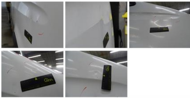
Sill outer R, Deformed / Strained, LI - Repair and paint (complete)
