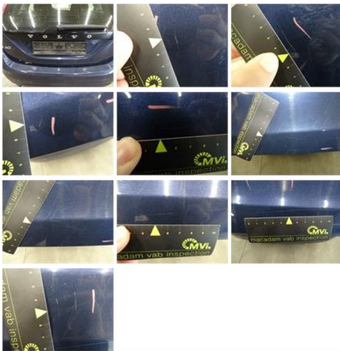
Door F L, Scratch(es), LI - Repair and paint (complete)
