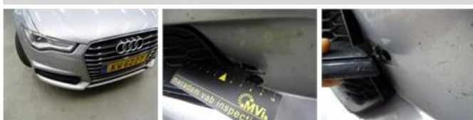
Bumper grille F R, Broken, E - Replace
