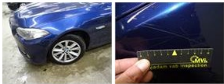
Bonnet, Scratch(es), LI - Repair and paint (complete)
