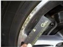
Alloy rim R L polished, Scratch(es), Acceptable
