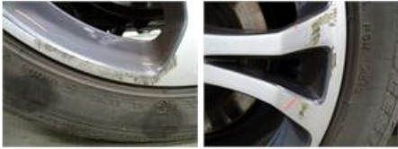
Alloy rim F L polished, Scratch(es), LI - Repair and paint (complete)
