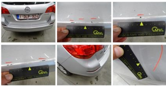
Trunk lid covering R, Scratch(es), Smart repair
