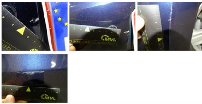
Roof, Scratch(es), LI - Repair and paint (complete)
