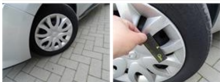
Wheel cover F R, Broken, E - Replace
