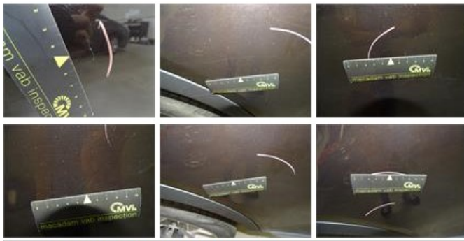
Door F L, Scratch(es), LI - Repair and paint (complete)
