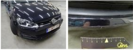
Bumper F, Scratch(es), It - Spot repair
