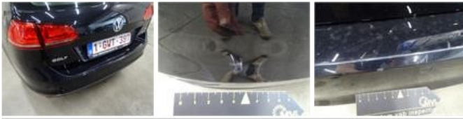
Bumper F, Scratch(es), It - Spot repair
