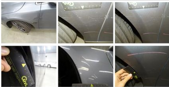
Wing R L, Dent(s) and scratch(es), LI - Repair and paint (complete)
