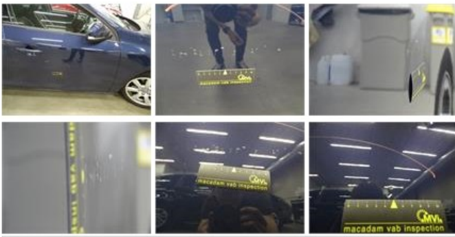
Door R R, Dent(s) and scratch(es), LI - Repair and paint (complete) 318,35
