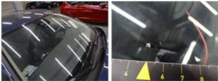
Door F L, Scratch(es), LI - Repair and paint (complete) 318,35
