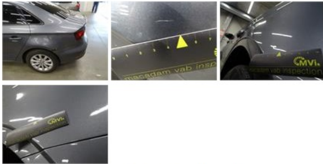
Tailgate, Chemical pollution, LI - Repair and paint (complete)
