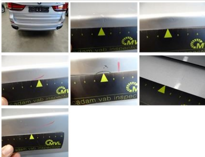
Sill outer R, Scratch(es), Acceptable
