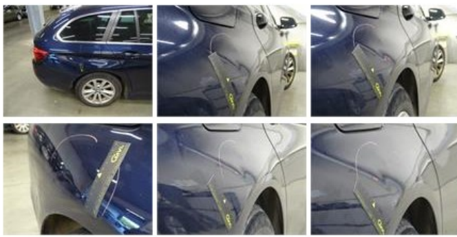
Door F R, Scratch(es), LI - Repair and paint (complete)
