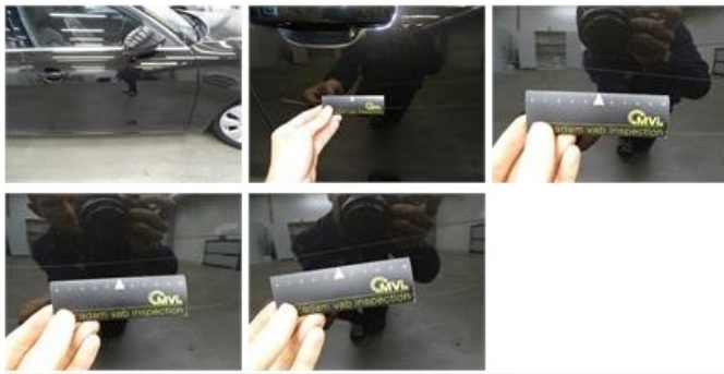
Wing R R, Scratch(es), LI - Repair and paint (complete)
