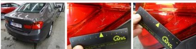
Rearlight R , Crack, E - Replace
