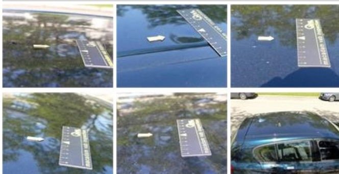
Sill trim L, Scratch(es), LI - Repair and paint (complete)
