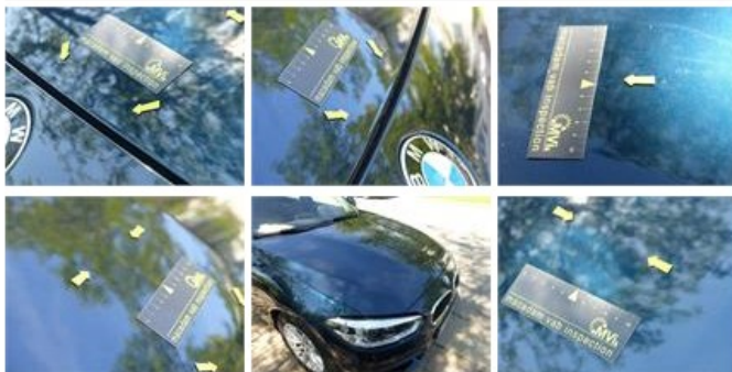
Roof, Dent(s), PDR - Paintless dent repair
