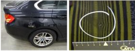
Wing R R, Dent(s) and scratch(es), LI - Repair and paint (complete)
