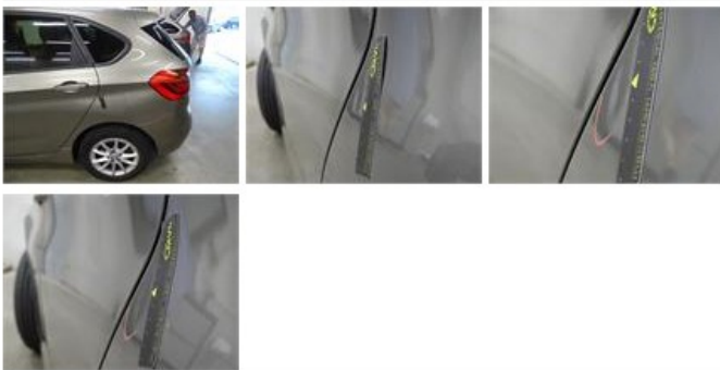
Door R R, Dent(s) and scratch(es), LI - Repair and paint (complete)
