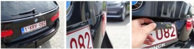
Tailgate, Dent(s), PDR - Paintless dent repair
